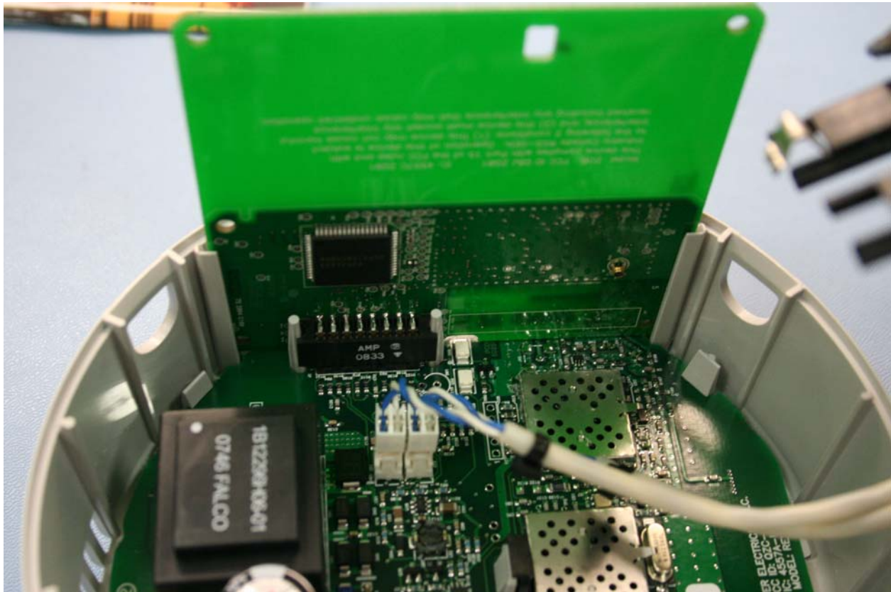
Close up View of a Production Model Installed in a “REX2” Power Meter (typical use for module)
