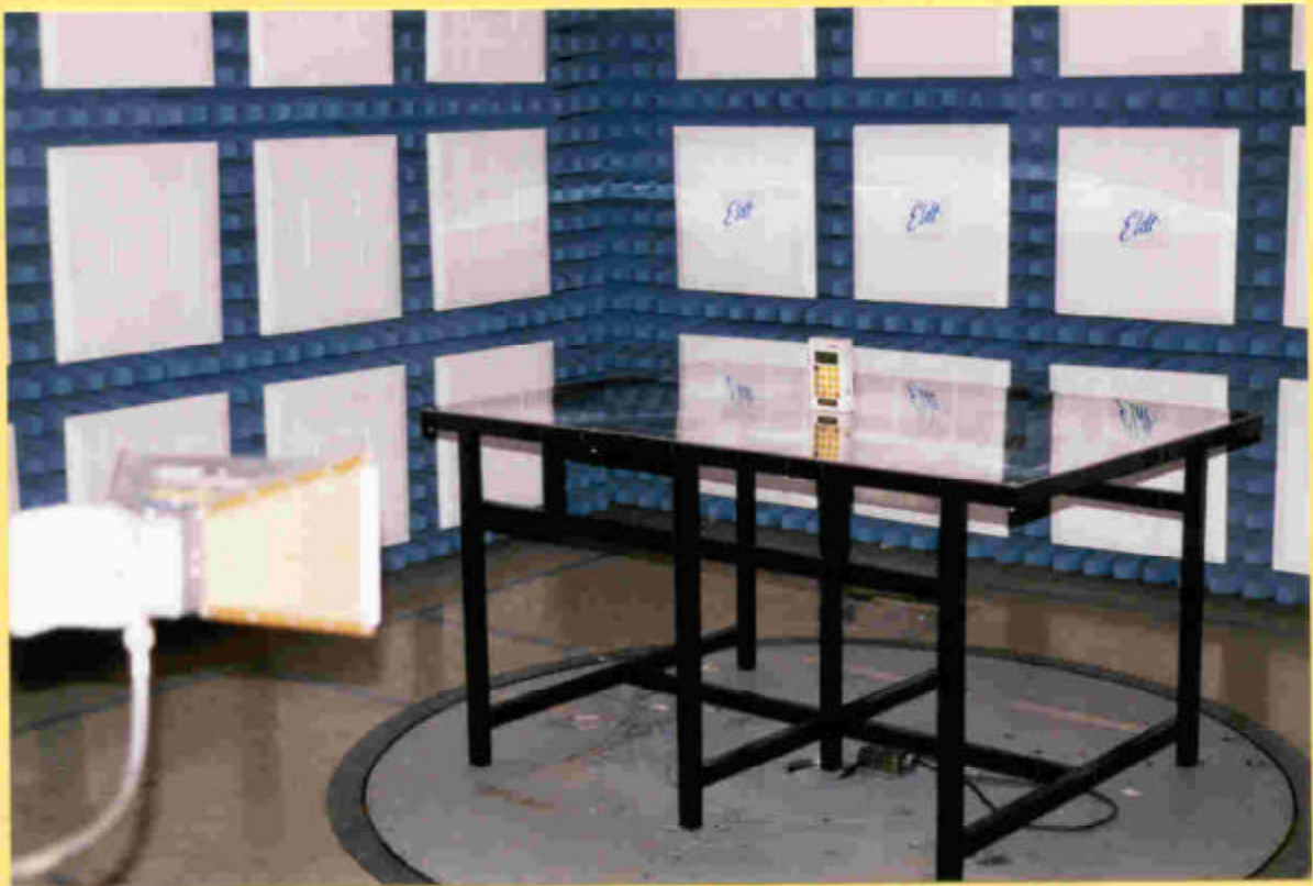
FIGURE 2D TEST SETUP FOR RADIATED EMISSIONS MEASUREMENTS MAXIMIZED FOR MEASUREMENT OF WORST CASE EMISSIONS VERTICAL POLARIZATION (ABOVE 1000MHZ)
