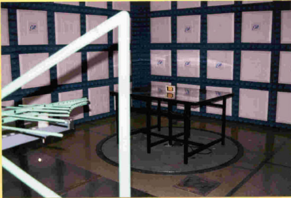
FIGURE 2A TEST SETUP FOR RADIATED EMISSIONS MEASUREMENTS MAXIMIZED FOR MEASUREMENT OF WORST CASE EMISSIONS HORIZONTAL POLARIZATION
