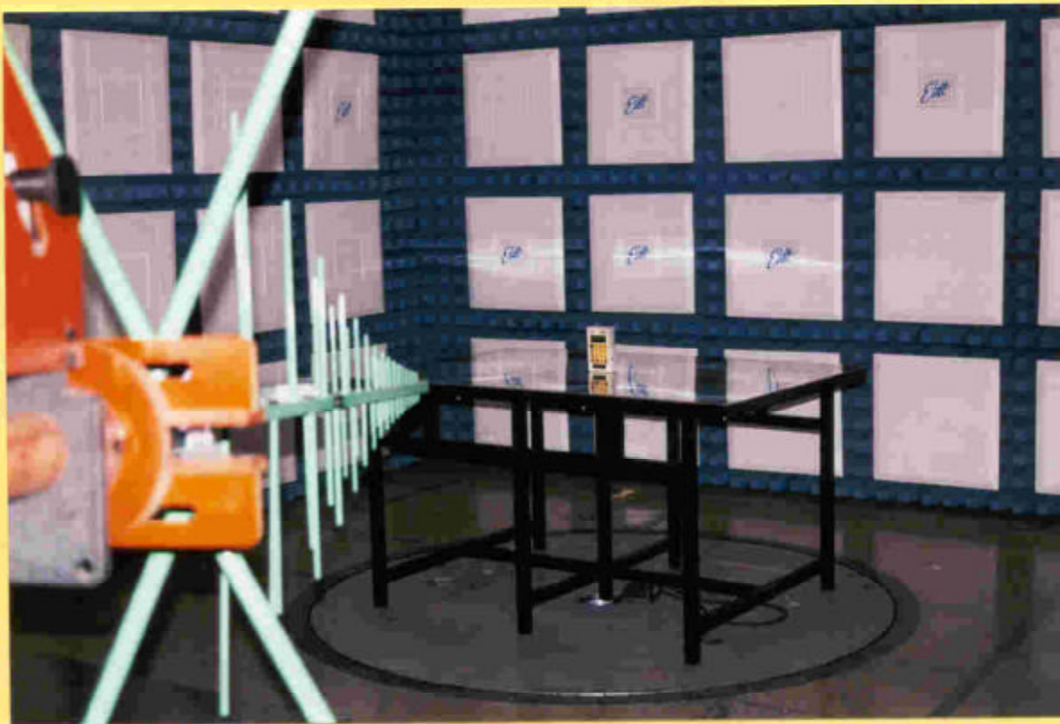
FIGURE 2B TEST SETUP FOR RADIATED EMISSIONS MEASUREMENTS MAXIMIZED FOR MEASUREMENT OF WORST CASE EMISSIONS VERTICAL POLARIZATION
