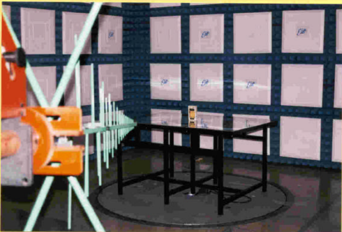
FIGURE 3B TEST SETUP FOR RADIATED EMISSIONS MEASUREMENTS MAXIMIZED FOR MEASUREMENT OF WORST CASE EMISSIONS VERTICAL POLARIZATION
