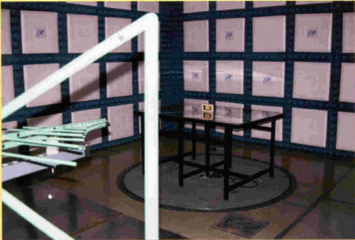
FIGURE 3A TEST SETUP FOR RADIATED EMISSIONS MEASUREMENTS MAXIMIZED FOR MEASUREMENT OF WORST CASE EMISSIONS HORIZONTAL POLARIZATION
