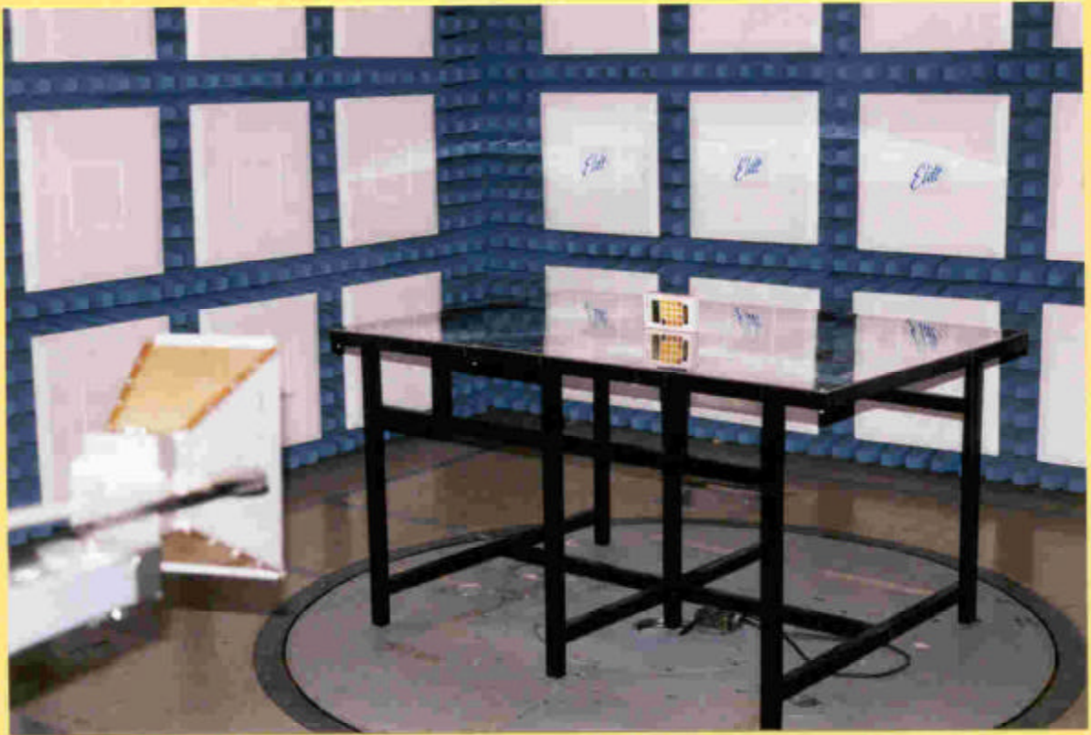
FIGURE 2C TEST SETUP FOR RADIATED EMISSIONS MEASUREMENTS MAXIMIZED FOR MEASUREMENT OF WORST CASE EMISSIONS HORIZONTAL POLARIZATION (ABOVE 1000MHZ)
