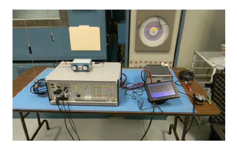
RTMI System with TX, RX Antennas, VGA Interactive Display, and GPS Receiver
