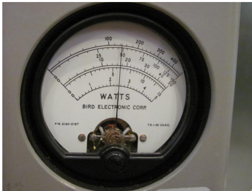
Power (rms) reading on a Bird Watt Meter
