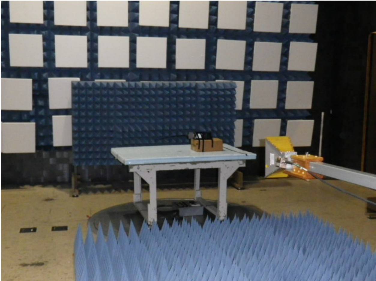
Figure 2: Typical Radiated Emissions at 3m – 1 GHz to 18 GHz.
