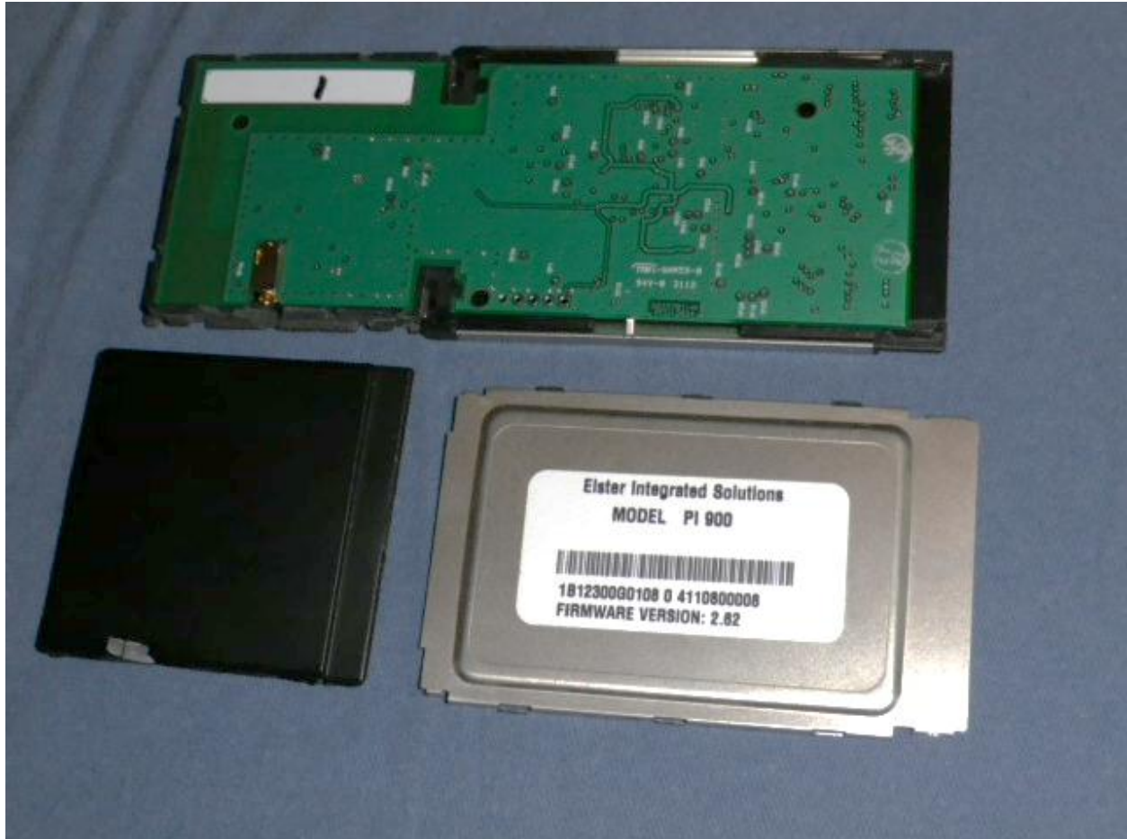
Figure 1: View of circuit board with transmitter inside the case
