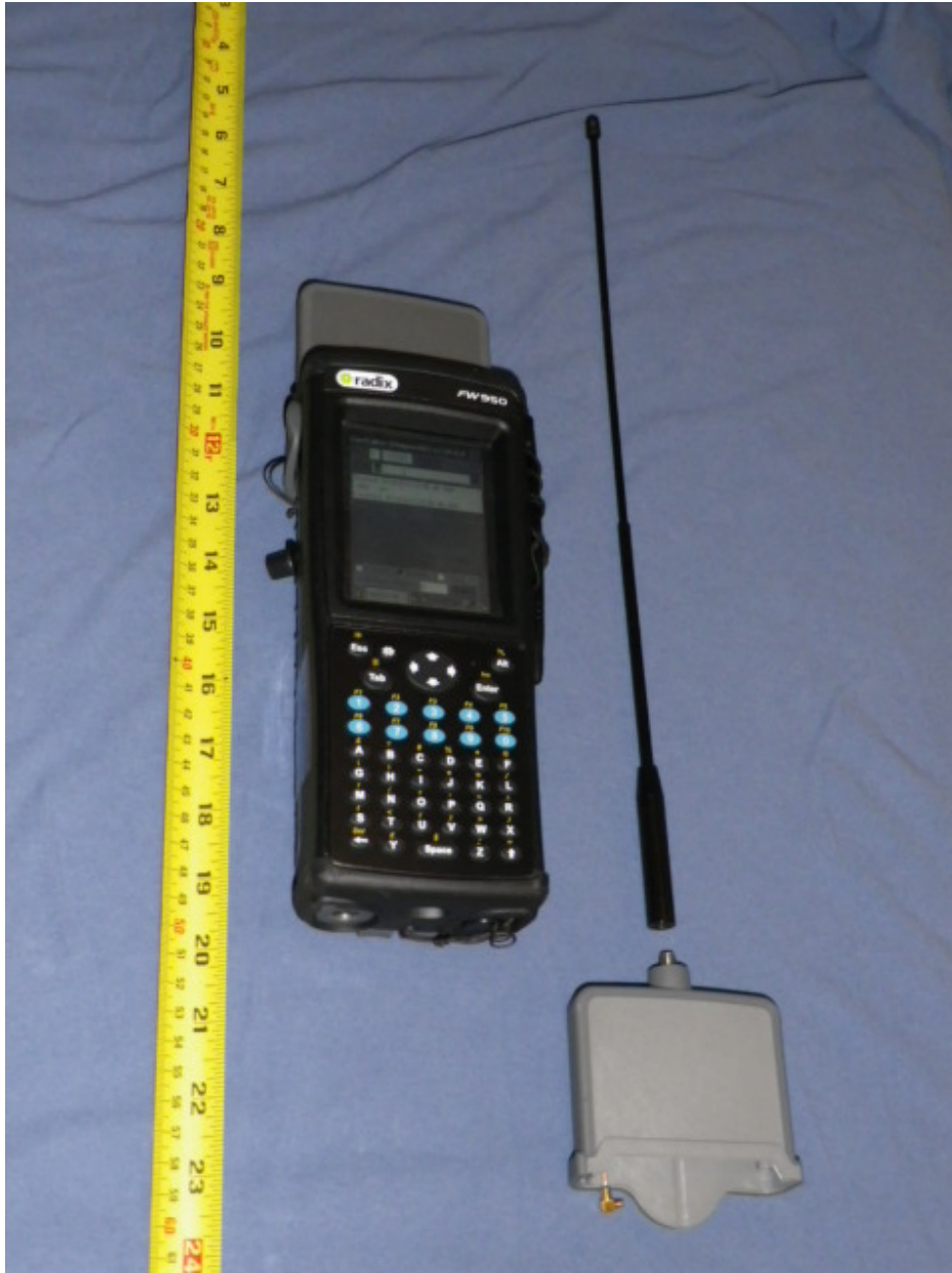
Figure 1: View of Model PI900W with internal antenna attached and the external antenna option.
