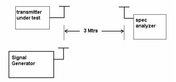
Method of Measurements: The tabulated data shows the results of the radiated field strength emissions test. The spectrum was scanned from 30 MHz to at least the tenth harmonic of the fundamental. This test was conducted per TIA/EIA STANDARD 603 using the substitution method.
