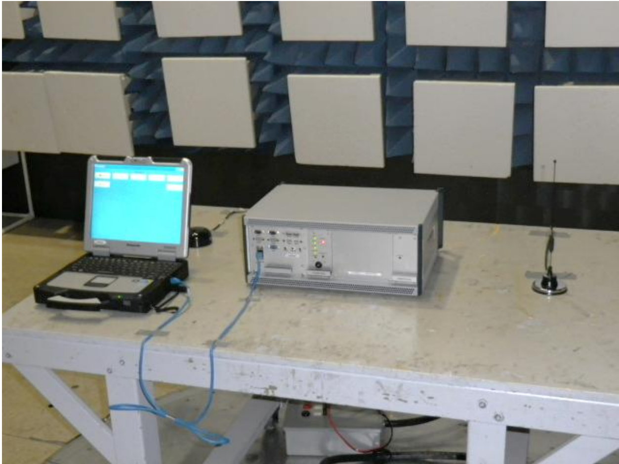
Figure 7 - Radiated Emissions Test Setup (Semi-Anechoic Chamber): 30 to 1000 MHz Shown with the laptop configuration (Worst case)
