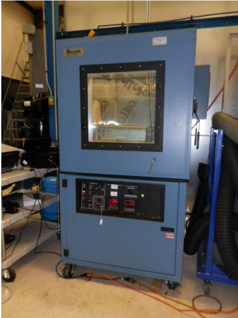
Figure 13: Extreme Temperature and Power Test setup – EUT inside Temperature Chamber.
