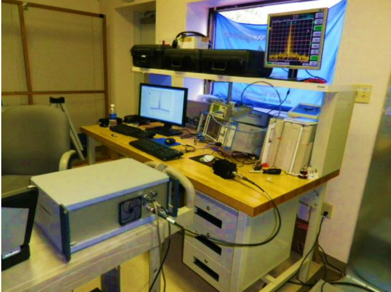
Figure 2: Rear View of Conducted RF Measurements.
