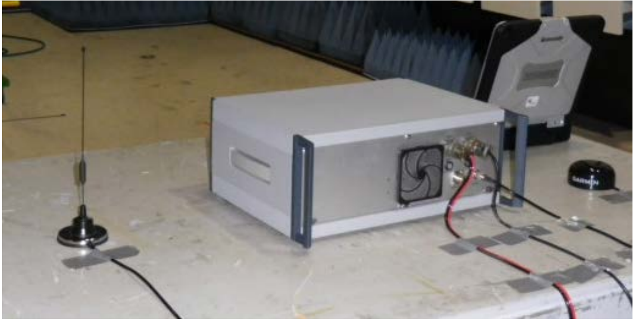
Figure 3: View of EUT showing external antennas with Computer Controller
