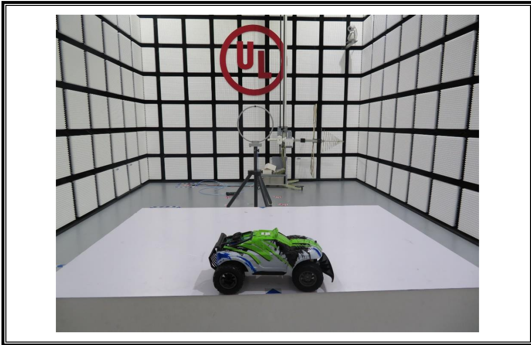
RADIATED RF MEASUREMENT SETUP (Below 30MHz)
