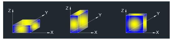
Note 1: For all radiated test, EUT in each of three orthogonal axis emissions had been tested, but only the worst case (X axis) data recorded in the report.
