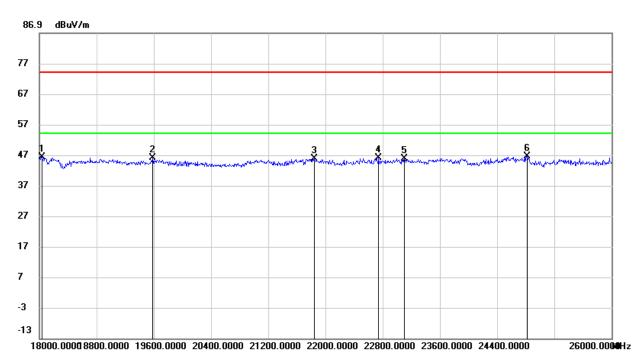
No. Frequency Reading Correct Result Limit Margin Remark (MHz) (dBuV) (dB/m) (dBuV/m) (dBuV/m) (dB) 18032.000 50.26 -3.93 46.33 74.00 -27.67 peak 2 19584.000 50.67 -4.64 46.03 74.00 -27.97 peak 21840.000 -5.93 45.66 74.00 3 51.59 -28.34 peak -5.74 45.94 74.00 4 22744.000 51.68 -28.06 peak 5 23104.000 51.35 -5.4745.88 74.00 -28.12 peak 46.58 6 24824.000 48.27 -1.69 74.00 -27.42 peak
