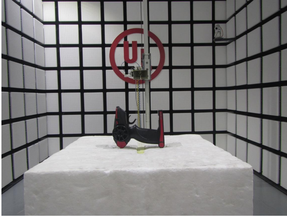
Radiated Disturbance Setup (Above 1 GHz – Z axis)
