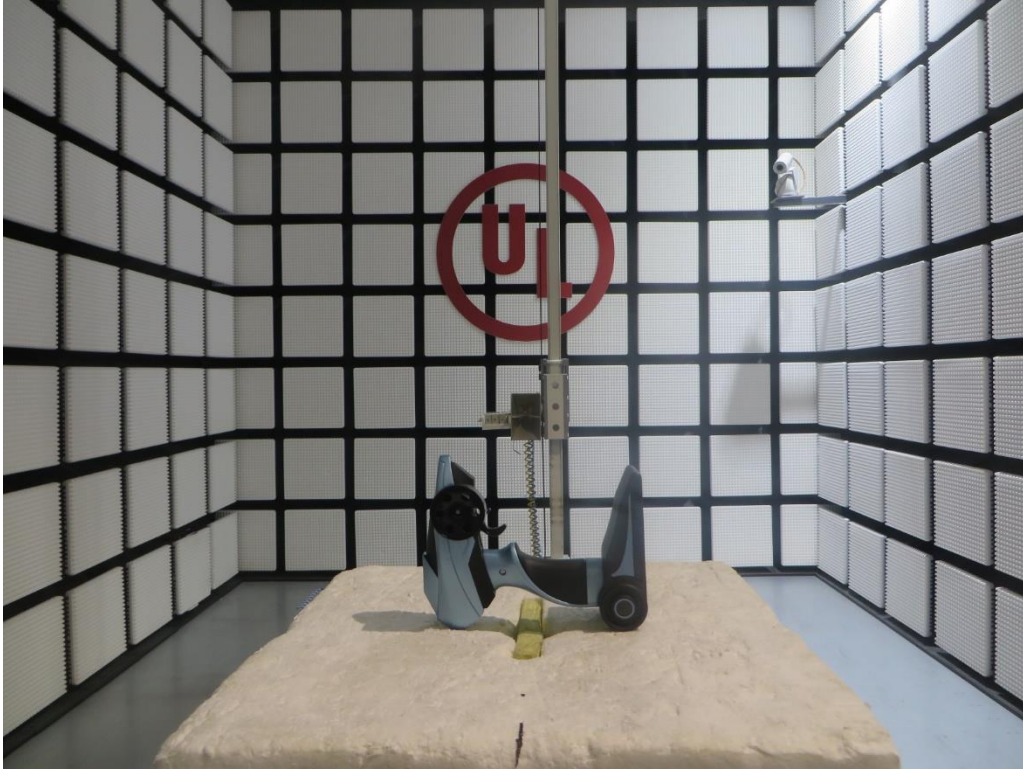
Radiated Disturbance Setup (Above 1 GHz-Z Axis)
