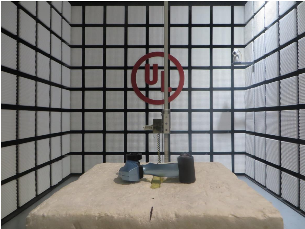
Radiated Disturbance Setup (Above 1 GHz-Y Axis)
