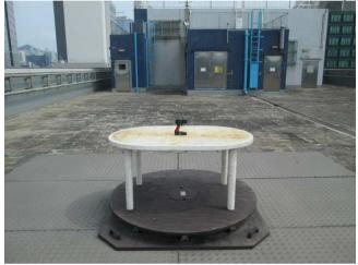
Measurement of Radiated Emission Test Set Up
