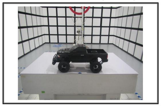
RADIATED RF MEASUREMENT SETUP (Below 30MHz)
