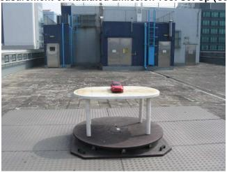
Measurement of Radiated Emission Test Set Up (Charger for Car)
