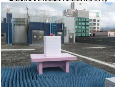
Measurement of Radiated Emission Test Set Up
