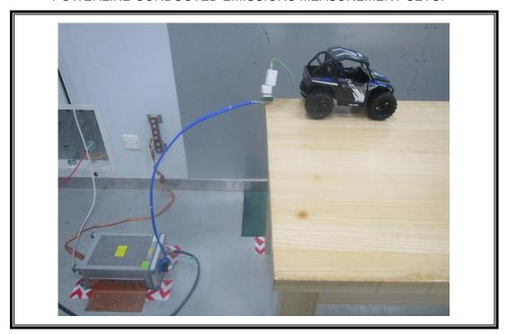
RADIATED RF MEASUREMENT SETUP (30MHz ~ 1 GHz)
