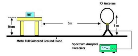
The setting of the spectrum analyzer
