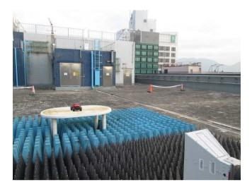
Measurement of Radiated Emission Test Set Up
