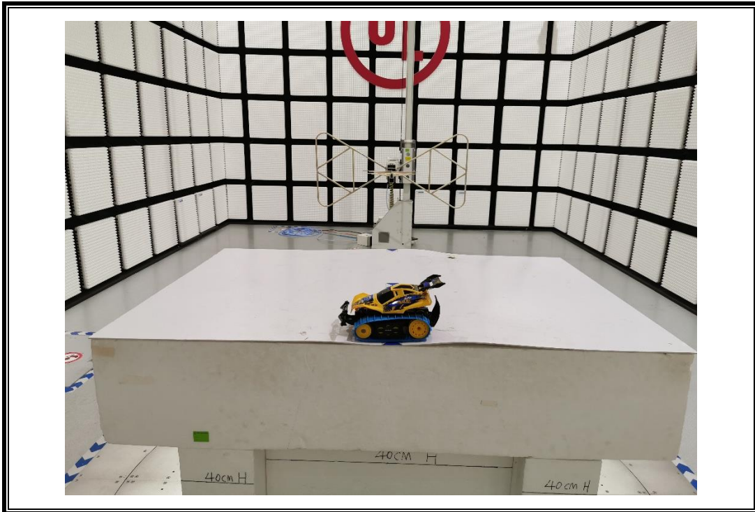
RADIATED RF MEASUREMENT SETUP (30MHz ~ 1 GHz)
