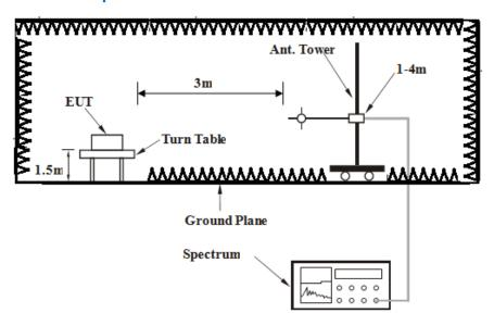
Note: For the actual test configuration, please refer to the attached file (Test Setup Photo).
