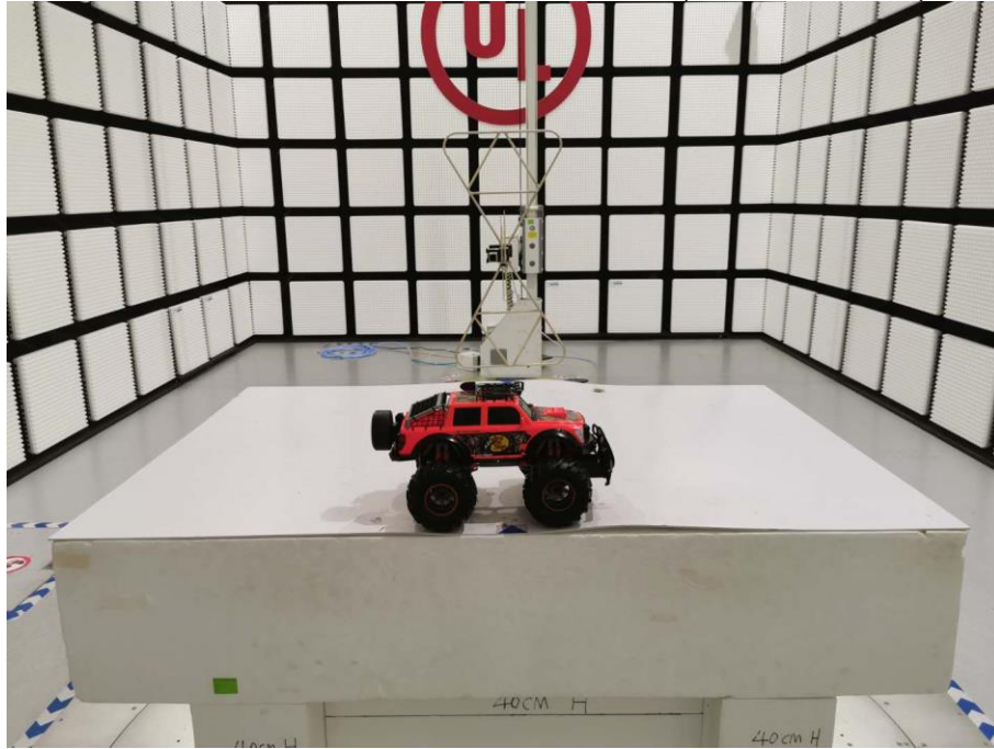
RADIATED RF MEASUREMENT SETUP (30MHz ~ 1 GHz)
