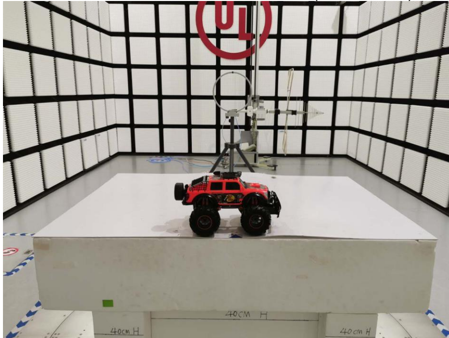
RADIATED RF MEASUREMENT SETUP (Below 30MHz)
