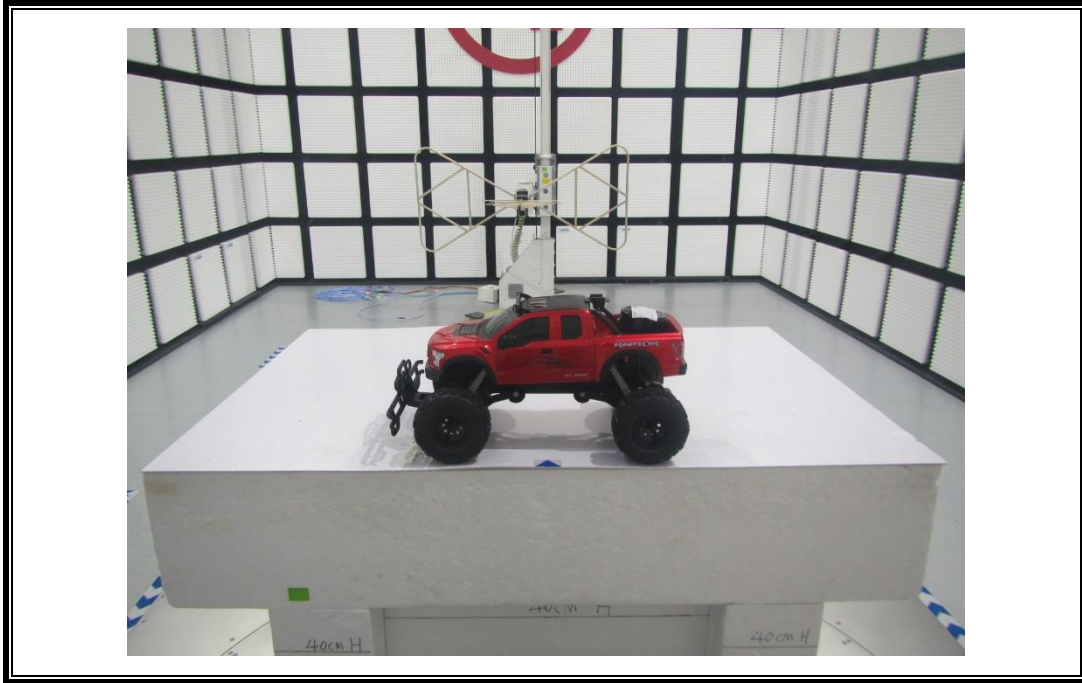
RADIATED RF MEASUREMENT SETUP (30MHz ~ 1 GHz)
