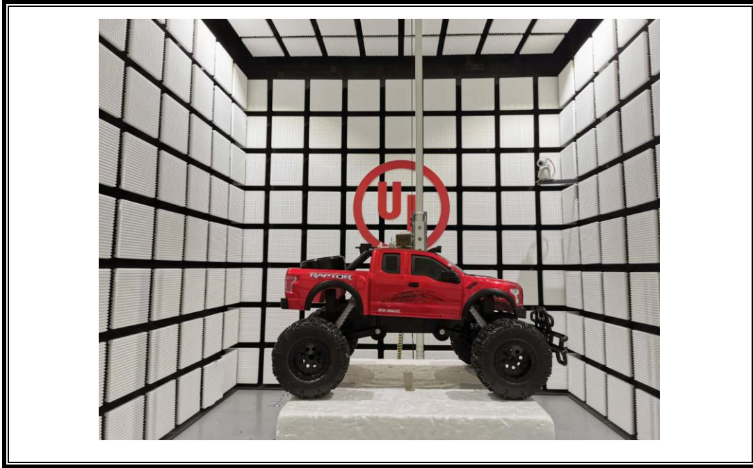
RADIATED RF MEASUREMENT SETUP (Above 1G – Y axis)
