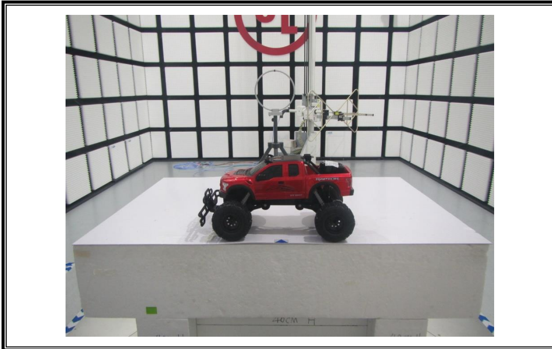
RADIATED RF MEASUREMENT SETUP (Below 30MHz)
