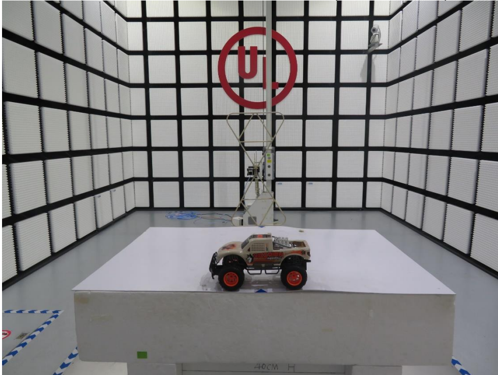
RADIATED RF MEASUREMENT SETUP (30MHz ~ 1 GHz)
