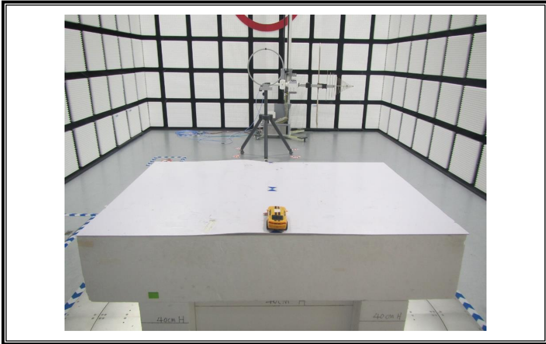
RADIATED RF MEASUREMENT SETUP (Below 30MHz)
