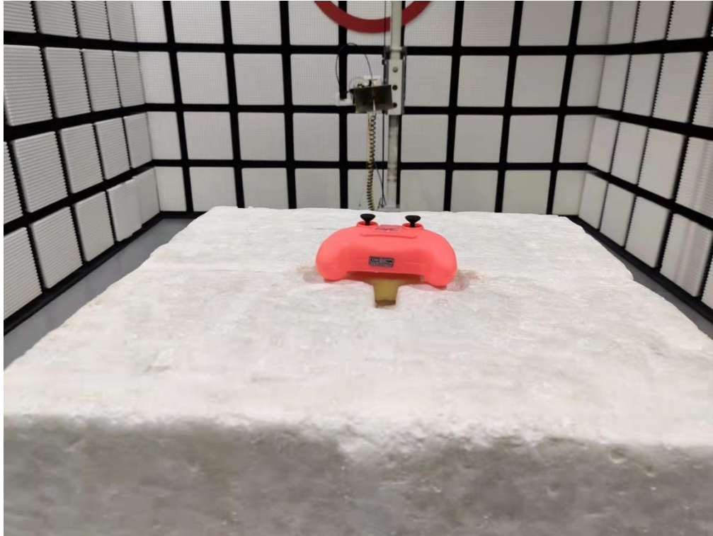
Radiated Disturbance Setup (Above 1 GHz – Y axis)
