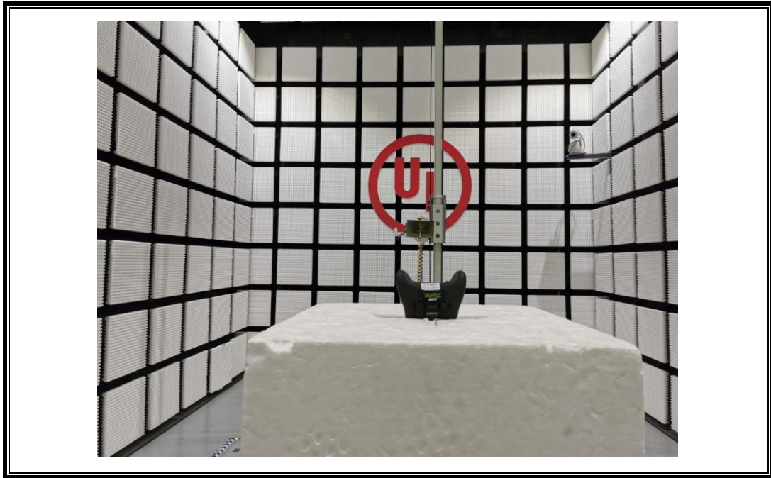
RADIATED RF MEASUREMENT SETUP (Above 1G – Z axis)
