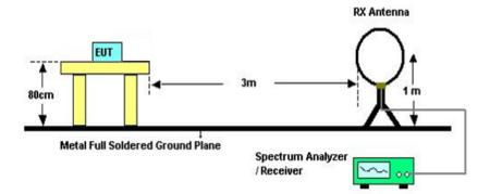
The setting of the spectrum analyzer
