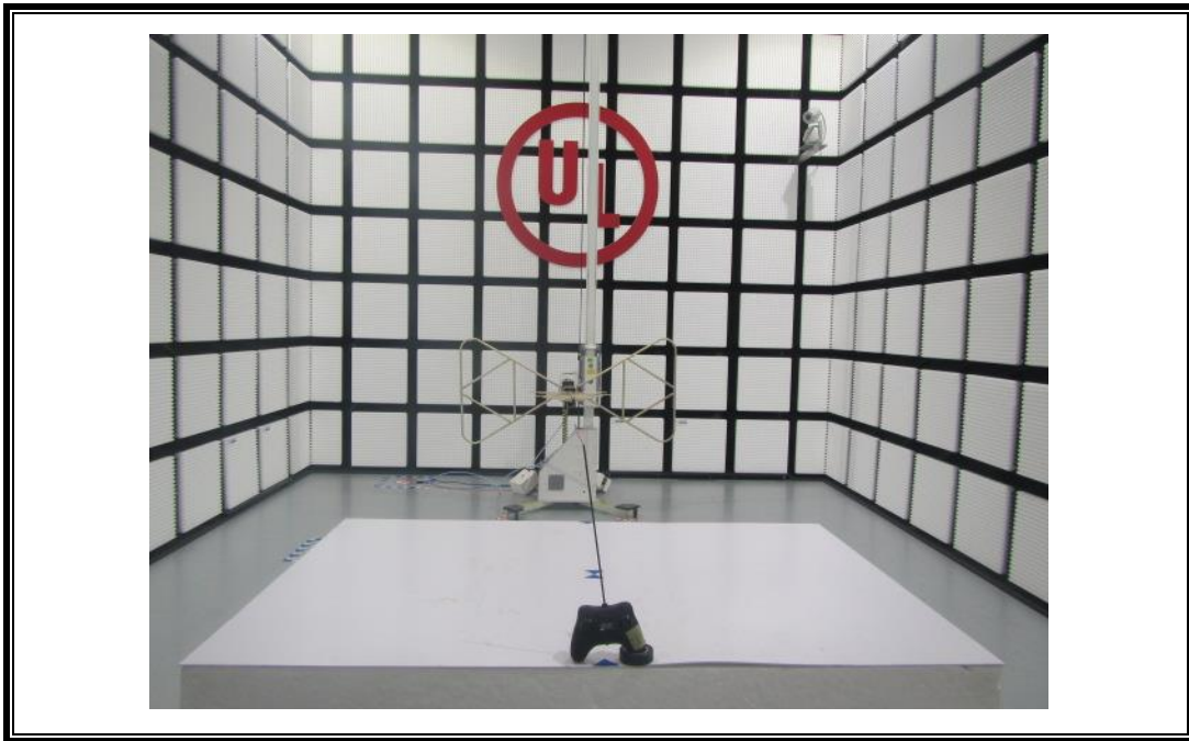
RADIATED RF MEASUREMENT SETUP (Above 30MHz and Below 1GHz – Z axis)
