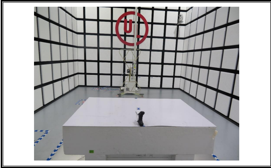
RADIATED RF MEASUREMENT SETUP (Above 30MHz and Below 1GHz – Z axis)
