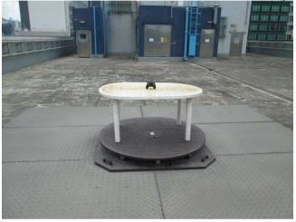
Measurement of Radiated Emission Test Set Up
