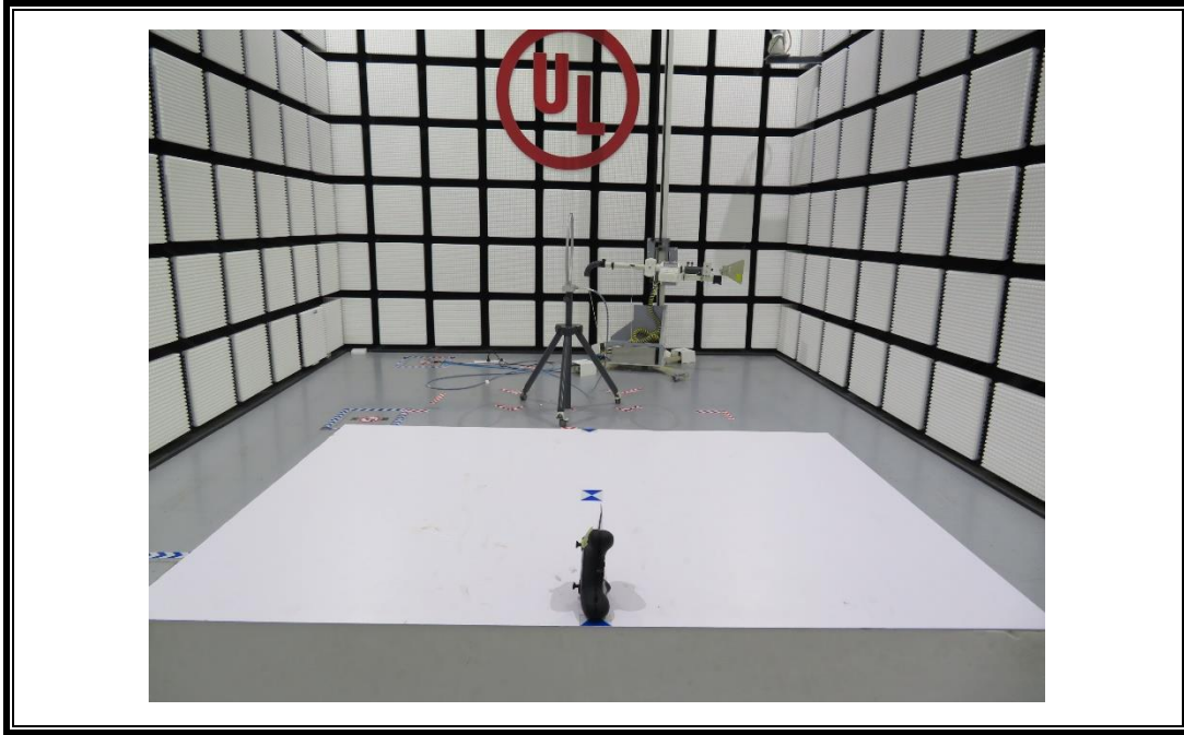
RADIATED RF MEASUREMENT SETUP (Below 30MHz – Z axis)
