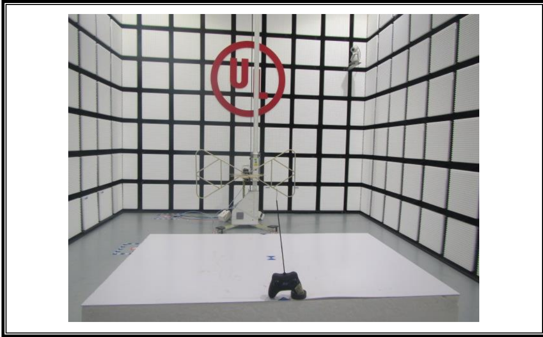
RADIATED RF MEASUREMENT SETUP (30MHz ~ 1 GHz)
