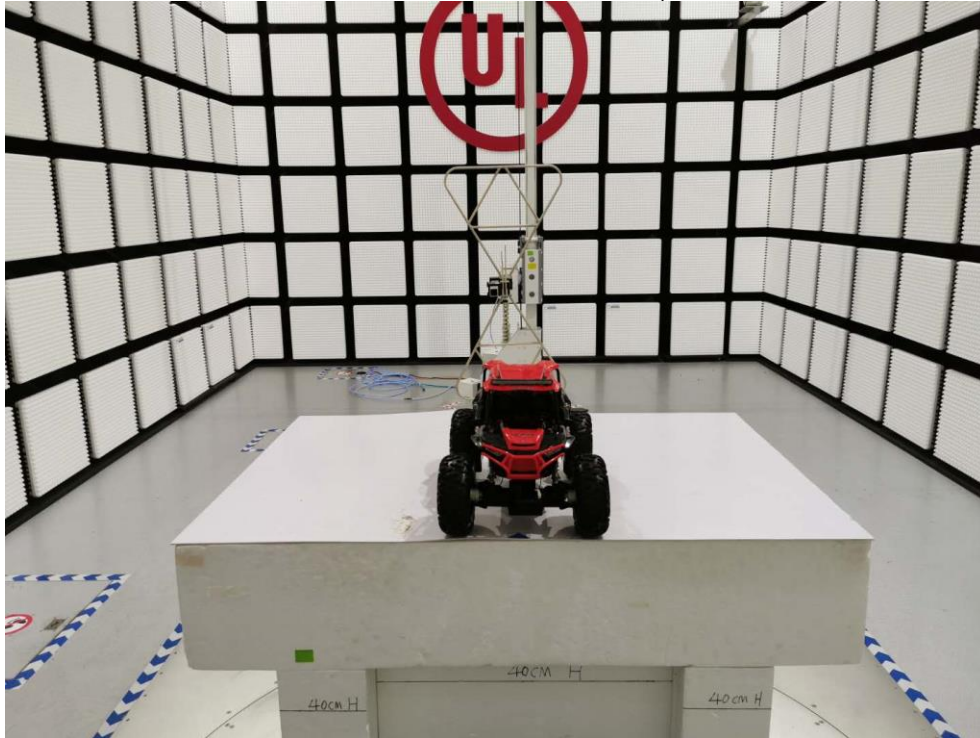
RADIATED RF MEASUREMENT SETUP (30MHz ~ 1 GHz)
