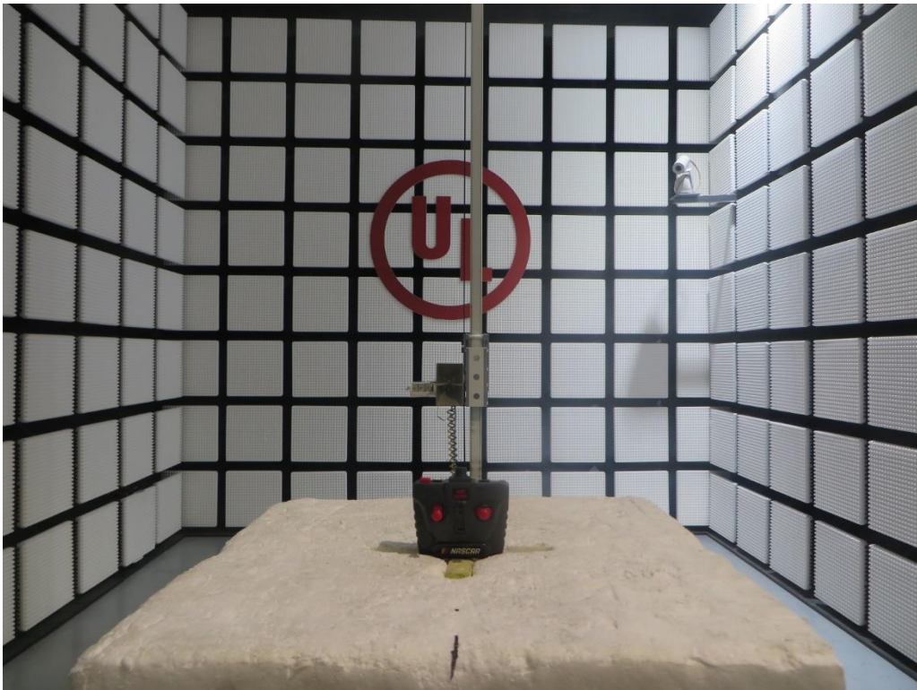
Radiated Disturbance Setup (Above 1 GHz-Y Axis)
