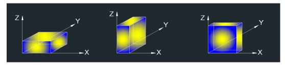
Note: For all radiated test, EUT in each of three orthogonal axis emissions had been tested, but only the worst case (X axis) data recorded in the report.
