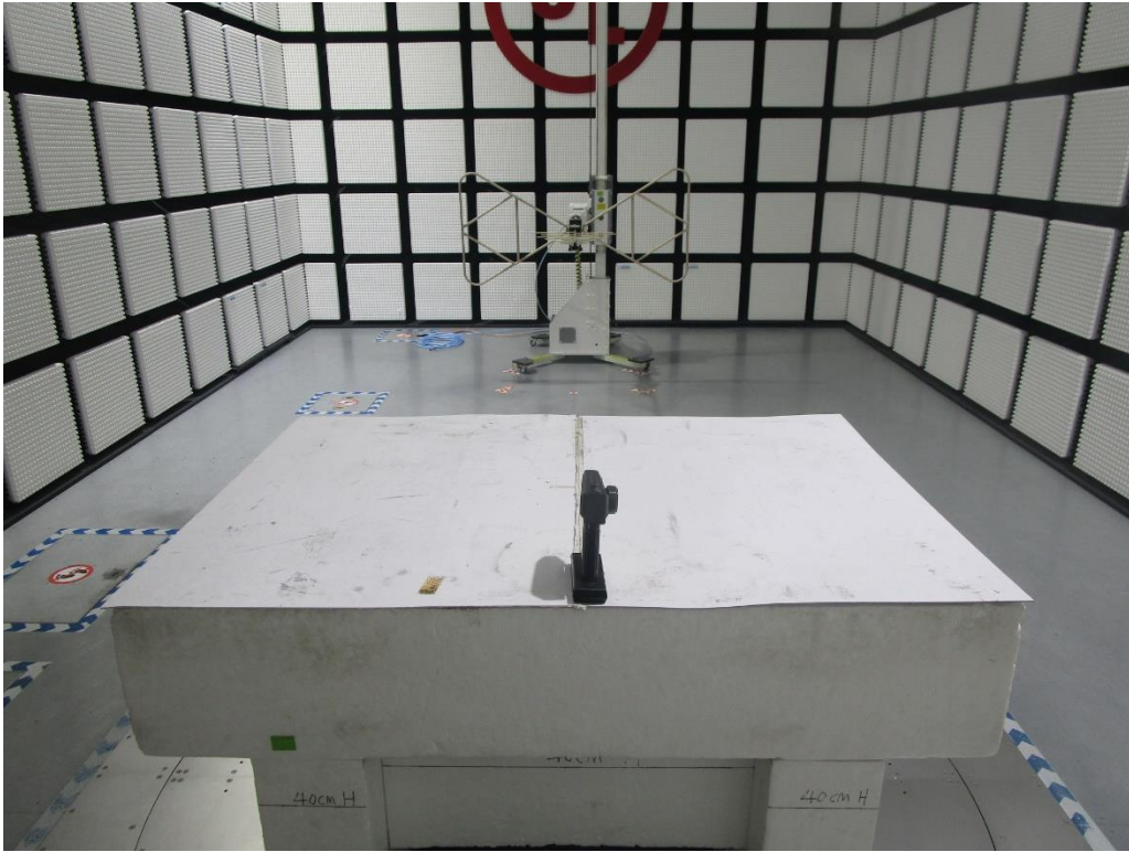
Radiated Disturbance below 30 MHz
