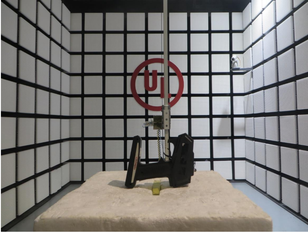
Radiated Disturbance Setup (Above 1 GHz-Z Axis)
