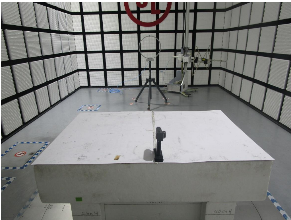
Radiated Disturbance below 30 MHz
