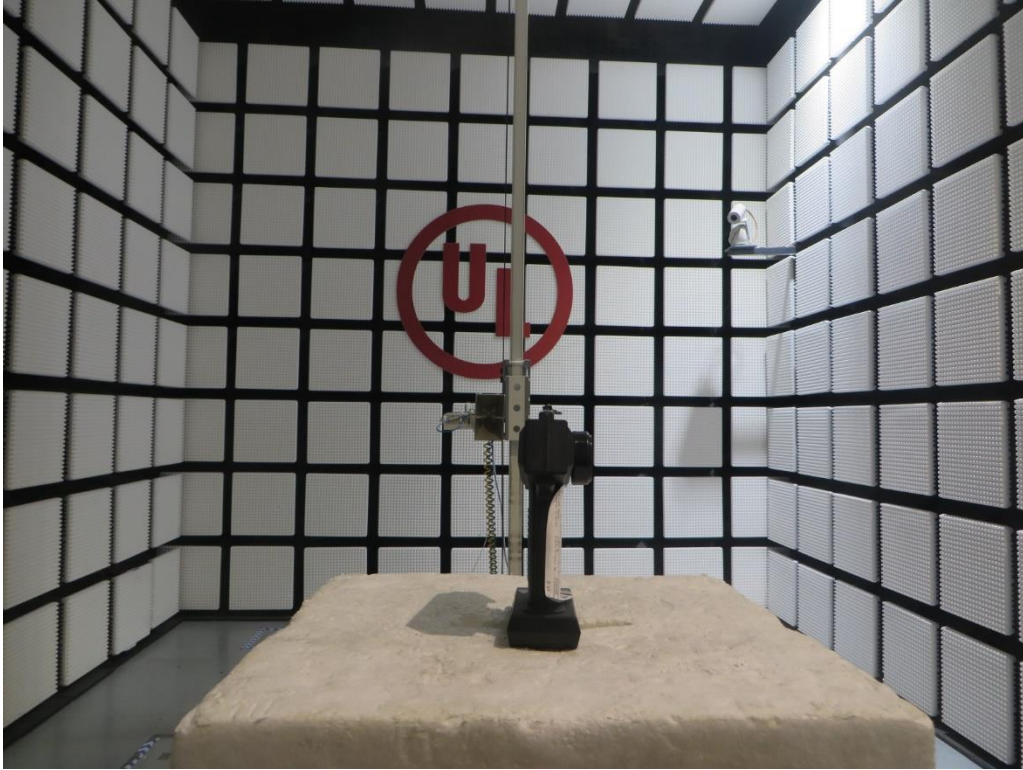
Radiated Disturbance Setup (Above 1 GHz-Y Axis)
