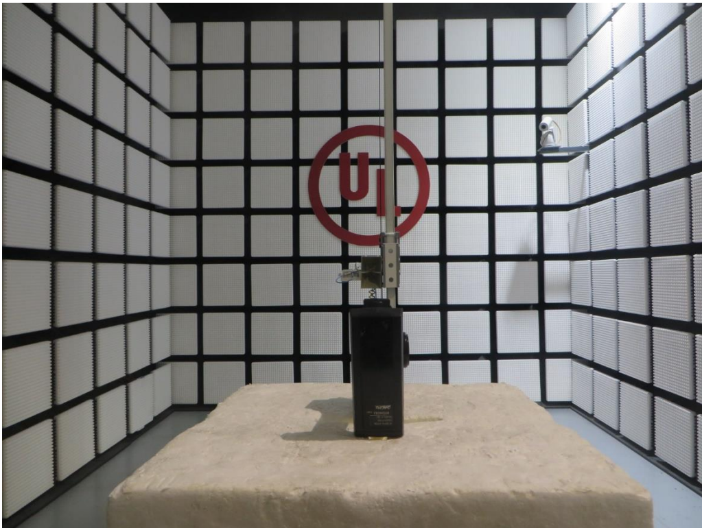
Radiated Disturbance Setup (Above 1 GHz-Y Axis)
