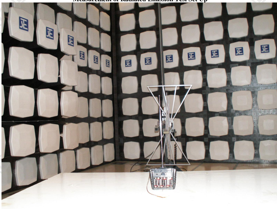
Measurement of Radiated Emission Test Set Up
