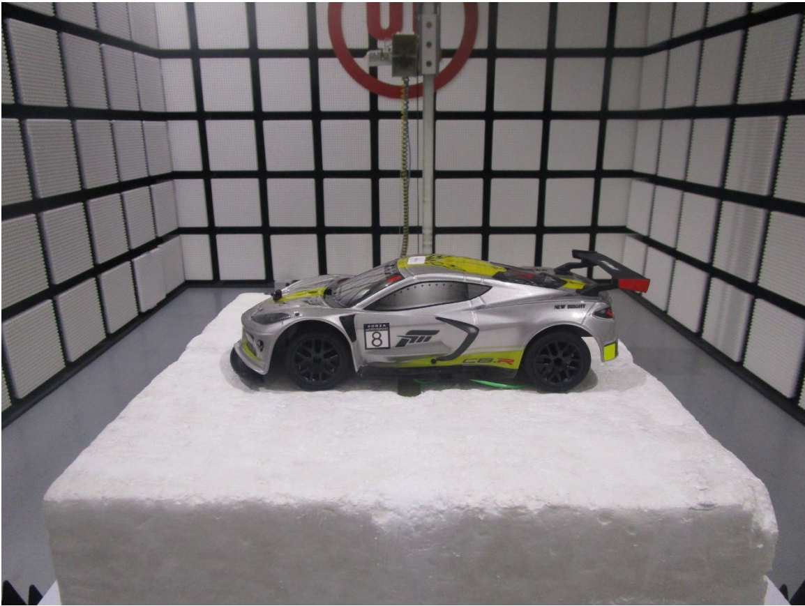
Radiated Disturbance Setup (Above 1GHz)
