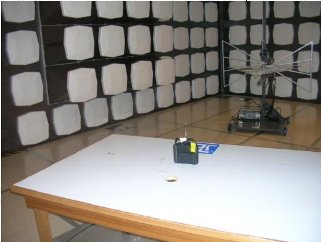
Measurement of Radiated Emission Test Set Up
