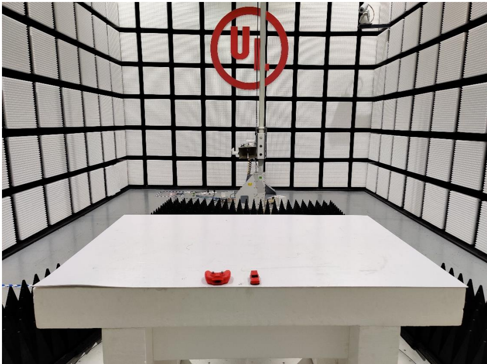
Radiated Emissions above 1GHz test setup photo
