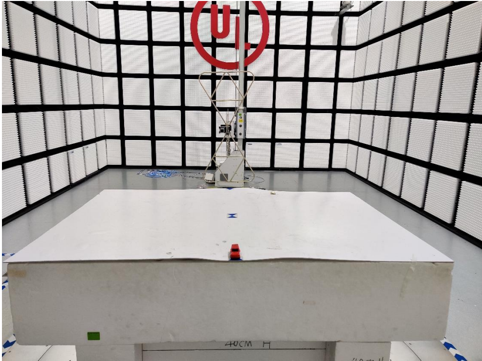
Radiated Emissions above 1GHz test setup photo
