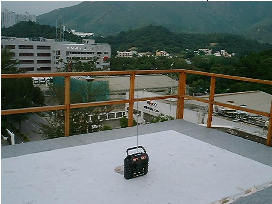
Measurement of Radiated Emission Test Set Up
