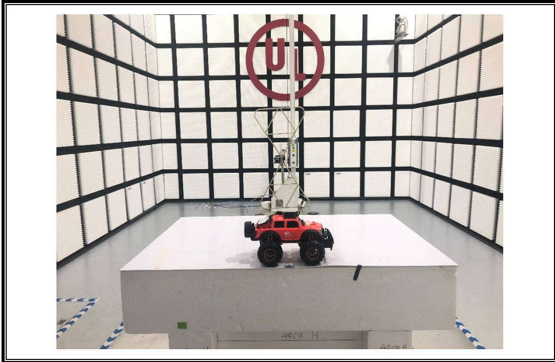
RADIATED RF MEASUREMENT SETUP (30MHz ~ 1 GHz)
