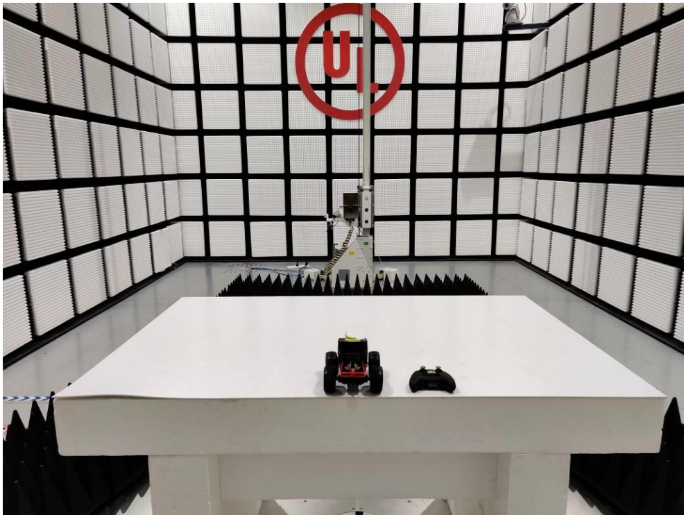
Radiated Emissions above 1GHz test setup photo
