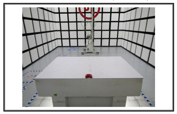
RADIATED RF MEASUREMENT SETUP (Below 30MHz)
