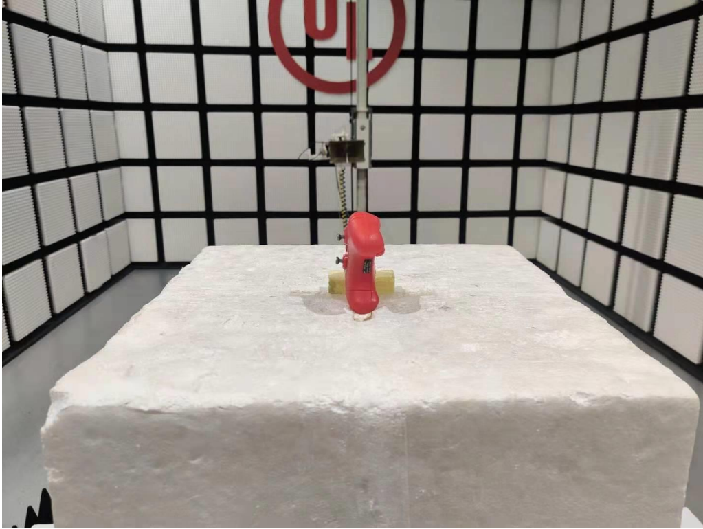
Radiated Disturbance Setup (Above 1 GHz – Z axis)
