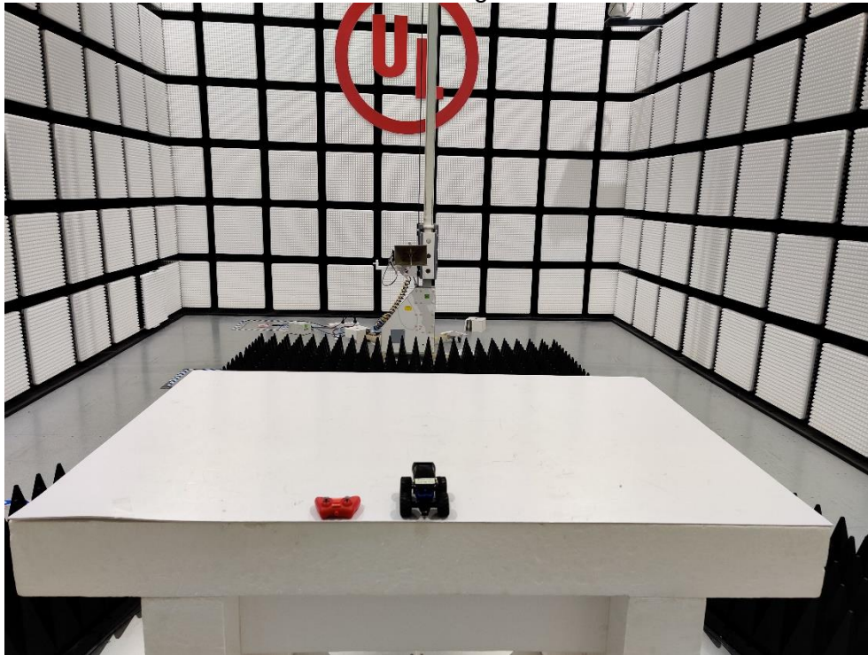
Radiated Emissions above 1GHz test setup photo
