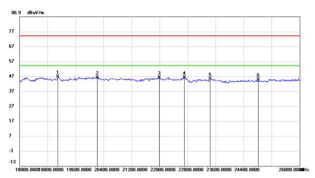
No. Frequency Reading Correct Result Limit Margin Remark (MHz) (dBuV) (dB/m) (dBuV/m) (dBuV/m) (dB) 19088.000 51.75 -4.9546.80 74.00 -27.20 peak 2 20224.000 51.16 -4.82 46.34 74.00 -27.66 peak -6.23 46.39 74.00 -27.61 3 21992.000 52.62 peak 46.27 -27.73 4 22704.000 52.02 -5.75 74.00 peak 45.34 5 23440.000 50.22 -4.88 74.00 -28.66 peak 6 24824.000 46.77 -1.69 45.08 74.00 -28.92 peak
