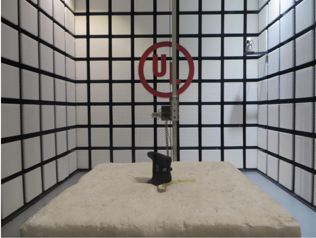
Radiated Disturbance Setup (Above 1 GHz-Z axis)
