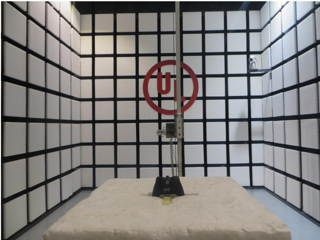
Radiated Disturbance Setup (Above 1 GHz-Y axis)
