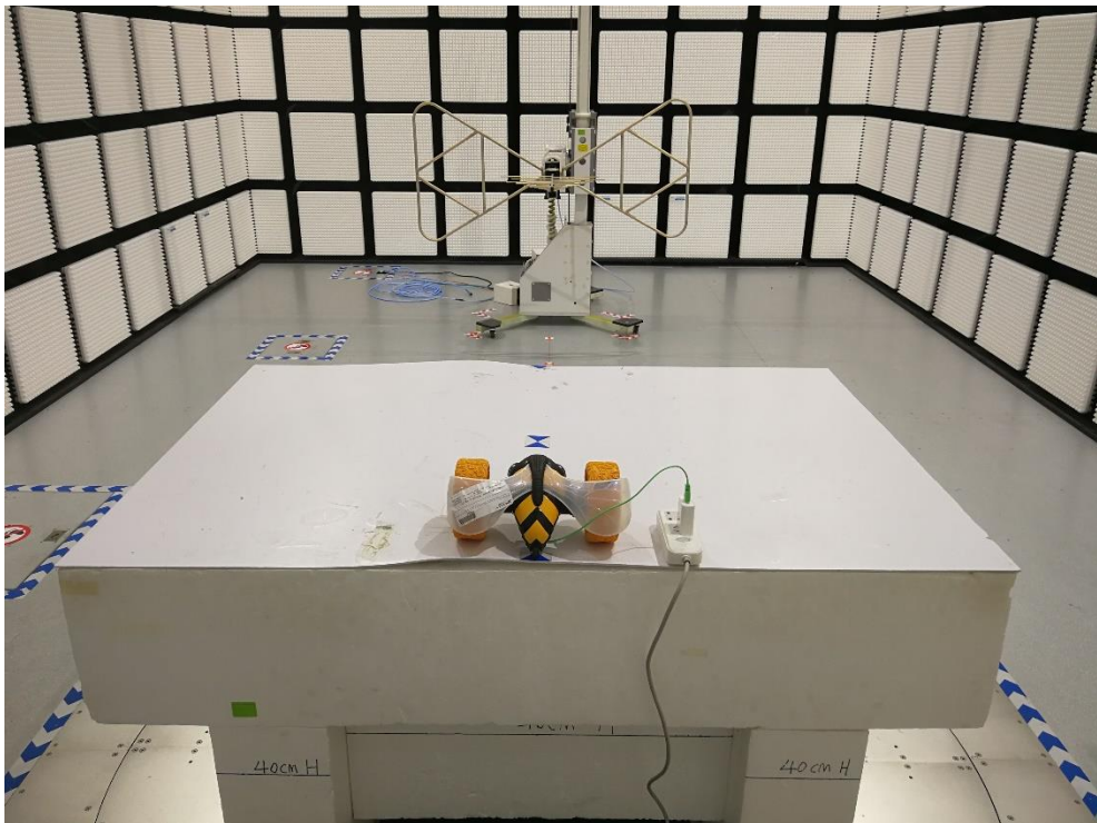
Radiated Emissions below 1GHz test setup photo
